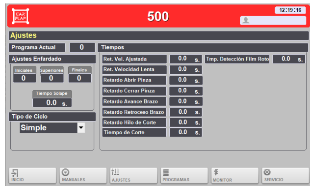
Photos: displays showing the wrapping cycles configuration and information about the machine status.
