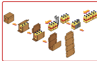
Infeed of the product at 90° and fitting.
