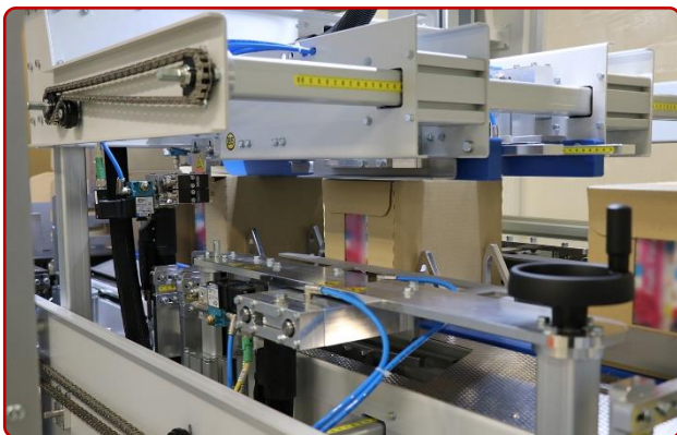
External flaps closing and square of the box pneumatically.
