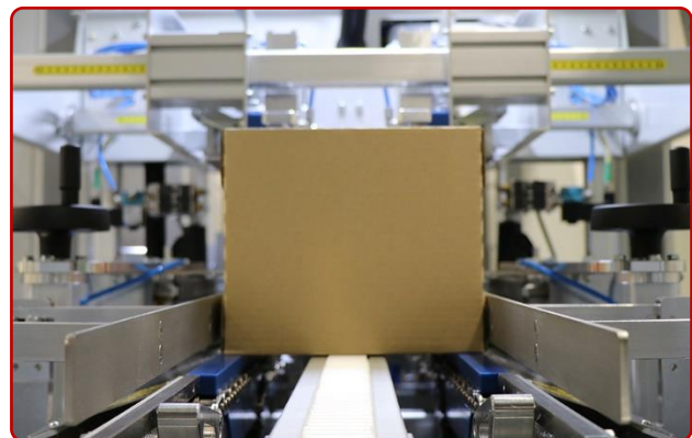
Infeed of the product in a line a packing of the product with the carton in a "U" position with a double movement of the pushing elements.
