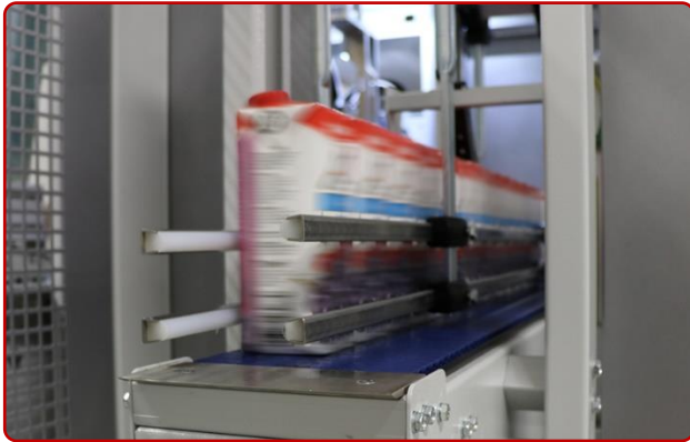
Infeed of the product in just 1 line. Optional: in 2- or 3-lines pattern.
