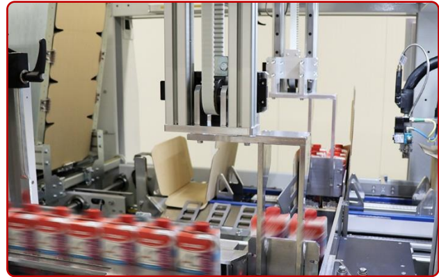
Infeed of the product in a line a packing of the product with the carton in a "U" position with a double movement of the pushing elements.
