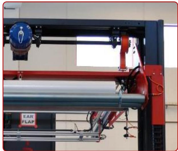
Elevation through slings, providing less noise and a simple maintenance without greasing.
