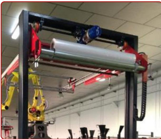
Motor brake for the elevation and descent of the arms which dispense the covering sheet.
