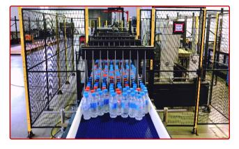
Side structure and railing to form the rails made of stainless Steel AISI304. A powered modular belt is used to transport the product, which has an "Intralox" design, controlled by an electronic speed inverter.
